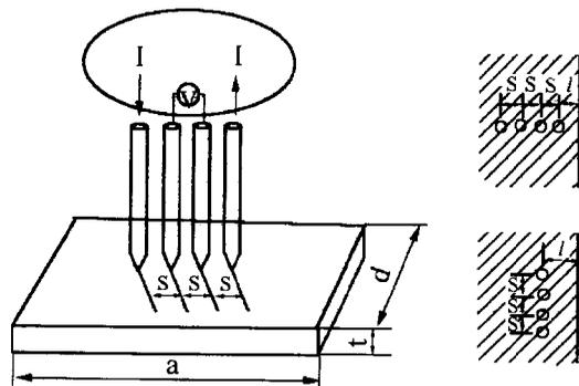
Fig. 1 Configuration of specimen boundary and 4 point probe
