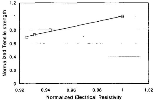
Fig. 6 Relation between normalized tensile strength and normalized electrical resistivity
