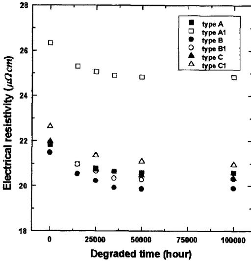
Fig. 3 Effect of degraded time on electrical resistivity
