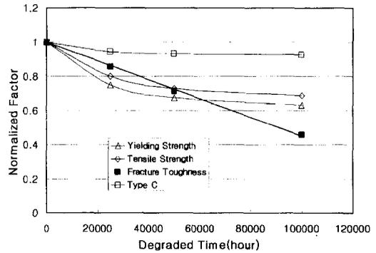
Fig. 5 Effect of normalized factors on degraded time
