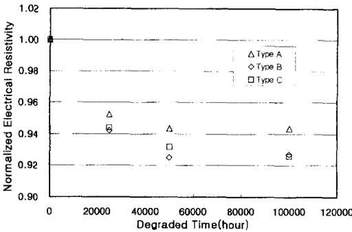
Fig. 4 Effect of normalized electrical resistivity on degraded time for different specimen type
